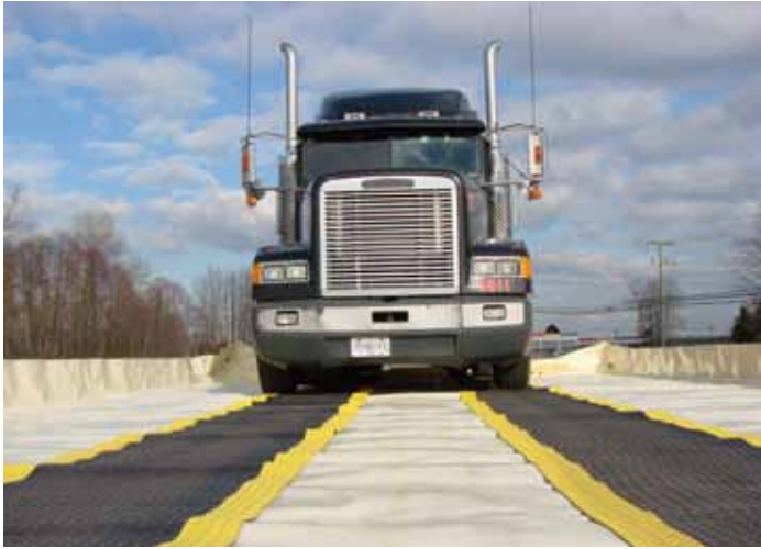
Optional track belting available to protect the berm from damage.
