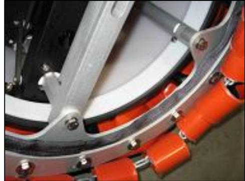
2. Collapse the IDS by pushing the hub into the bucket.
