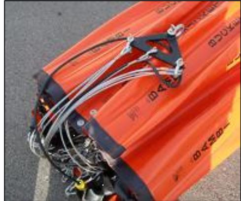
7. Roll the bucket into a bundle and wrap with straps supplied.
