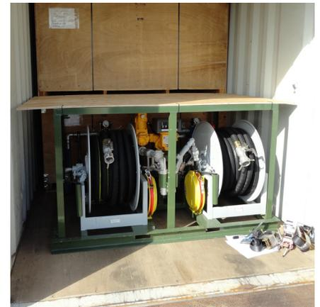
Various nozzles are provided to enable filling of ground vehicles, tanker trucks or small aircraft. Portable secondary containment is provided for each mechanical skid. Flexible hoses are provided to connect the entire system together via manifolds built onto each filling and dispensing skid.
