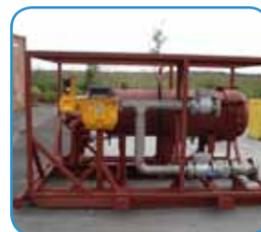
A robust pumping/filtering equipment ensures fuel is clean before the fuel reaches the Arctic King™ tanks.
