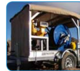
Portable fuel transfer trailers like this one enable bulk fuel transfer into tanker trucks for delivery throughout the mine.
