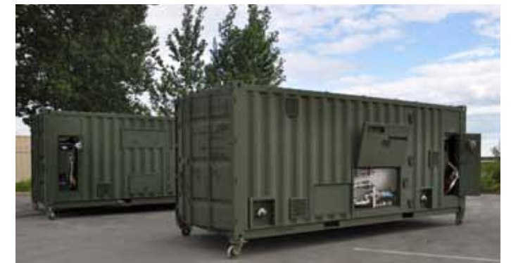
SEI fuel storage and transfer system deployed at Cold Lake, Alberta. System contained: four 24, 000 USG (90,800 L) Arctic King Tanks , a 185 USGPM (700 LPM) electric powered High Pressure Aviation Refueling System (HPARS) , Insta-Berm (framed supported) and a RainDrain rain water filtration system.
