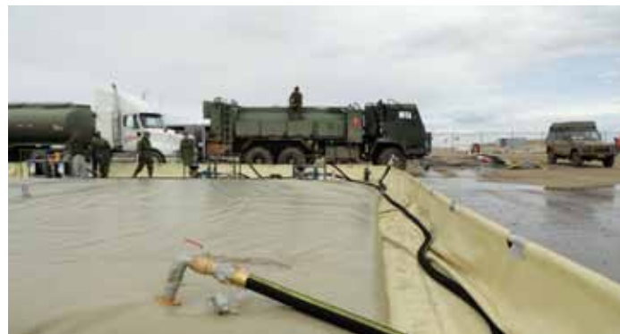
SEI fuel storage and transfer system deployed at Cold Lake, Alberta. System contained: four 24, 000 USG (90,800 L) Arctic King Tanks , a 185 USGPM (700 LPM) electric powered High Pressure Aviation Refueling System (HPARS) , Insta-Berm (framed supported) and a RainDrain rain water filtration system.
