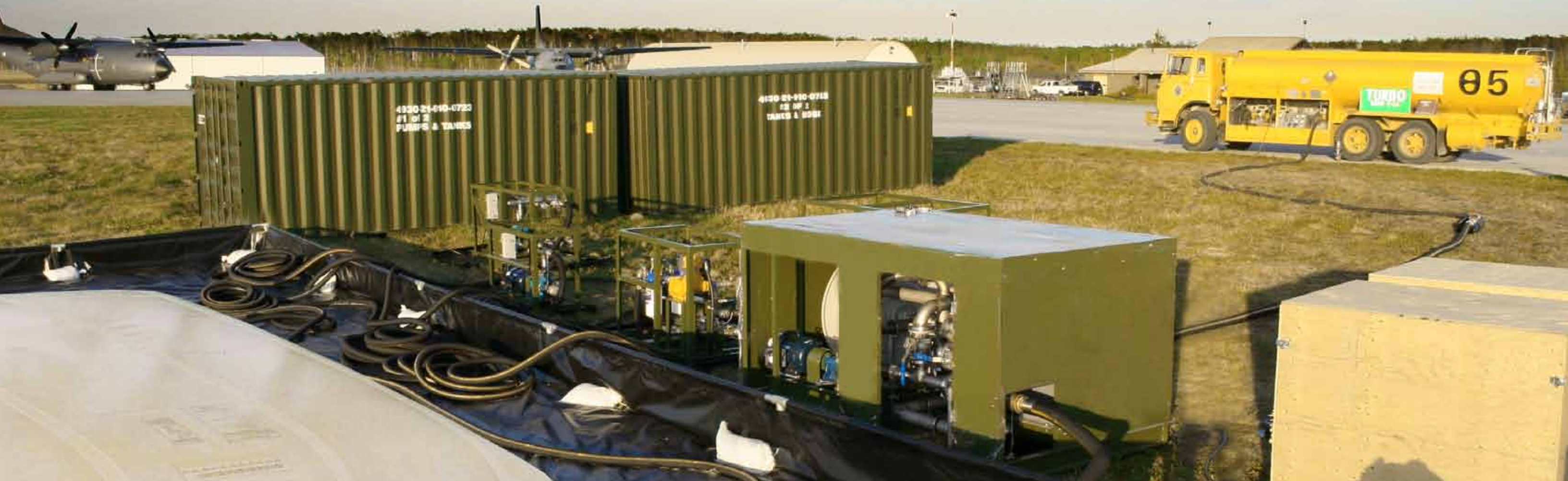
SEI fuel storage and transfer system deployed at Cold Lake, Alberta. System contained: four 24, 000 USG (90,800 L) Arctic King Tanks , a 185 USGPM (700 LPM) electric powered High Pressure Aviation Refueling System (HPARS) , Insta-Berm (framed supported) and a RainDrain rain water filtration system.
