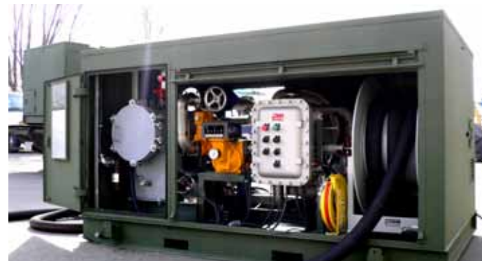
SEI fuel storage and transfer system deployed at Cold Lake, Alberta. System contained: four 24, 000 USG (90,800 L) Arctic King Tanks , a 185 USGPM (700 LPM) electric powered High Pressure Aviation Refueling System (HPARS) , Insta-Berm (framed supported) and a RainDrain rain water filtration system.
