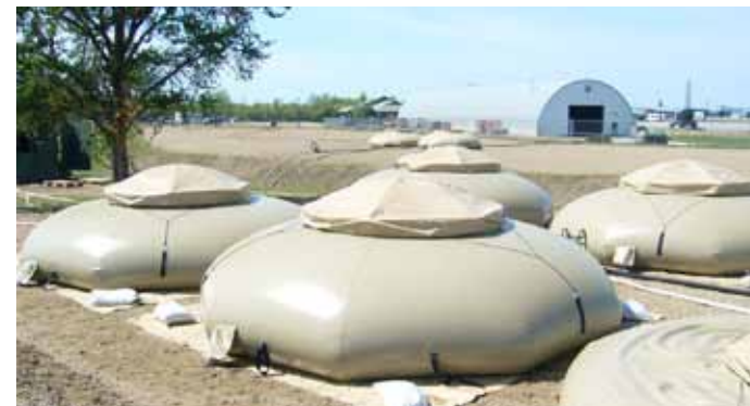
SEI fuel storage and transfer system deployed at Cold Lake, Alberta. System contained: four 24, 000 USG (90,800 L) Arctic King Tanks , a 185 USGPM (700 LPM) electric powered High Pressure Aviation Refueling System (HPARS) , Insta-Berm (framed supported) and a RainDrain rain water filtration system.
