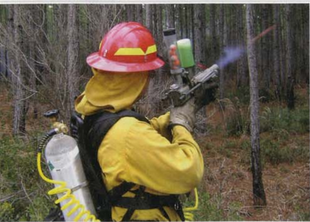
Above: National Interagency Prescribed Fire Training Center photo of Pyroshot HS handheld launcher being tested. The Pyroshot launches Dragon Eggs over water bodies and into fuels that are inaccessible by foot. Photo taken Feb. 28, 2008, Tate's Hell State Forest, Florida.
