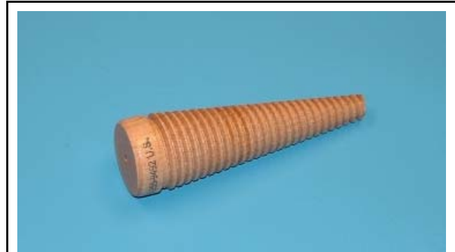
Wooden screws can be used to temporarily repair minor leaks.
