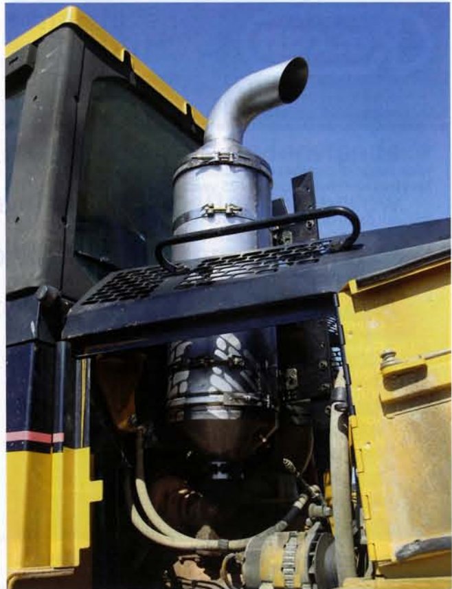
Eco Waste Solutions' ThermoCat features a fully automated diesel particulate filter system.
