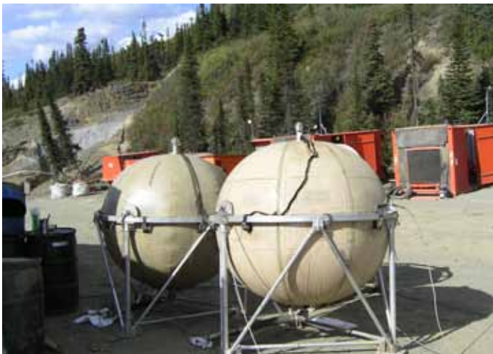
The rigid aluminum frame protects the aircell during transport.
