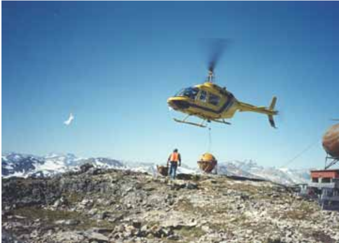
Fuel-Easy is specially designed for transferring fuel using a helicopter.
